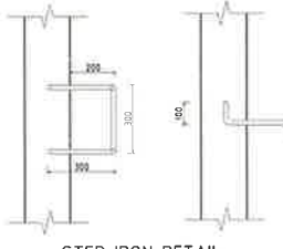
STEP IRON DETAIL NOT TO SCALE STEP IRON OF 20mm GALVANIZED STEEL MADE TO SHAPE AND DIMENSIONS SHOWN AND PLACED AT 300 CENTRES AND STAGGERED HORIZONTALLY FOR PITS DEEPER THAN 150mm
